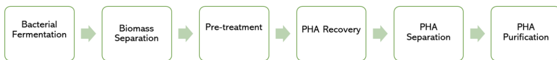
Figure 9. Schematic representation of the steps involved in PHA production, from the upstream section (bacterial fermentation) to the downstream. The downstream portion is, mainly, divided in five phases. Adapted from (Kosseva & Rusbandi, 2018).
